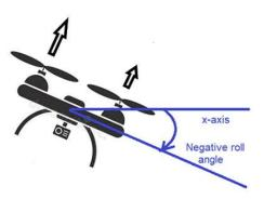
When the drone is at rest, it has a roll angle of zero. A positive roll angle corresponds to a leftward tilt, and a negative roll angle corresponds to a rightward tilt.
