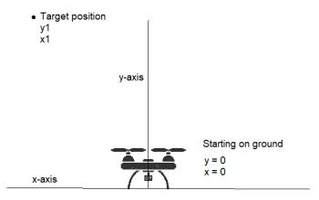
For this we need to tilt the drone sideways, which is called Roll (measured in angle). This is done by varying the thrust (or rpm) between the rotors of the Drone. In a Dual Rotor Drone, if thrust on the right side is higher, the Drone will roll left. If thrust on the left side is higher, then the Drone will roll right.
