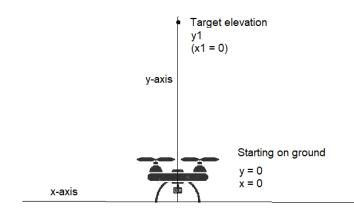
We have to induce a certain rpm (rotations per minute) equally in both the rotors. As the rpm of its rotors increase, they push the air down and this exerts a net upward force (thrust) on the Drone.
