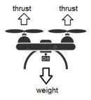
When this force equals the weight of the Drone, it starts to hover. Increasing the rpm beyond this point will lift the Drone up. To reach a certain elevation within some limited time, the thrust has to be sufficiently high. But as the drone nears the target, we have to start reducing the thrust until it is back equal to its weight ideally right at the target elevation. There, we have to maintain this thrust in order for it to hover for the desired period.
