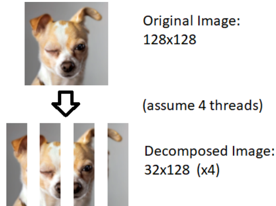
Figure 2: Example decomposition of input. Notice that data will be balanced among threads.
