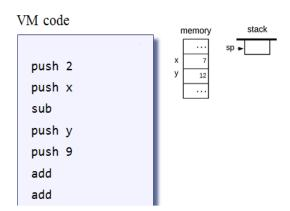
3. Stack Logical Commands: Again, what the state of the stack and memory after the following VM code is executed. Where will the stack pointer (sp) end up, if it originally begins at address 256? Please illustrate the stack after every VM command has been executed.
